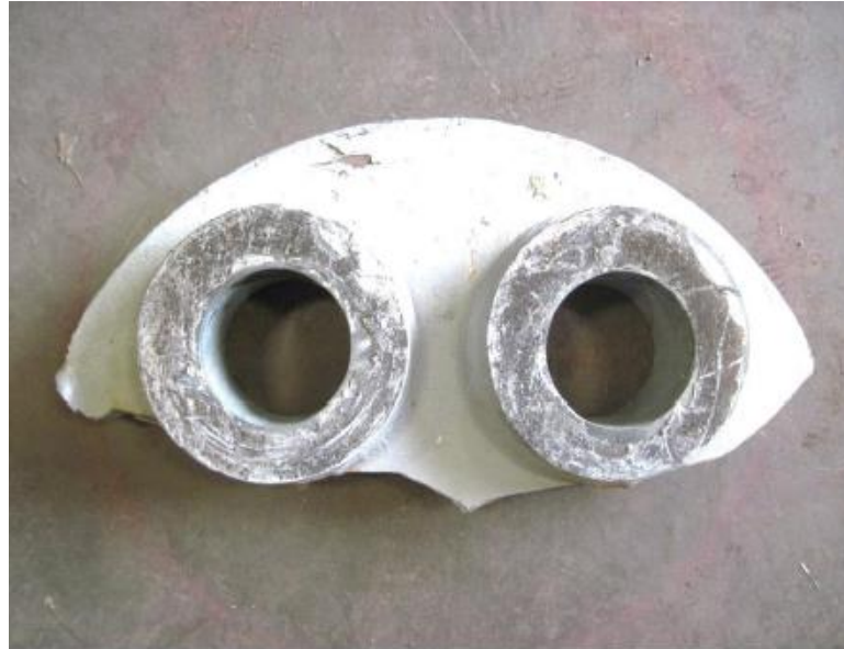
Segment of Cable Diaphragm Plate 9 that separated from the pylon following plate fracture.
