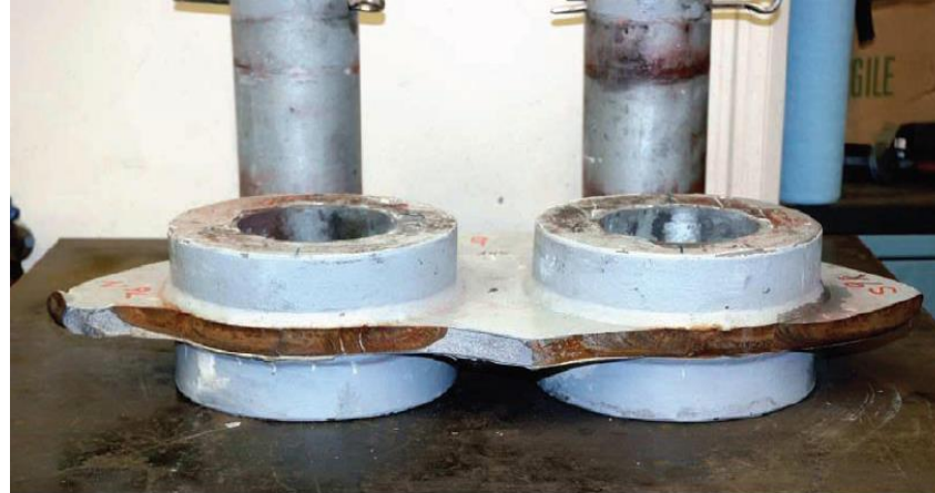
View of fracture surface of Cable Diaphragm Plate 9 showing crack growth from weld toes of ring plates and end welds
